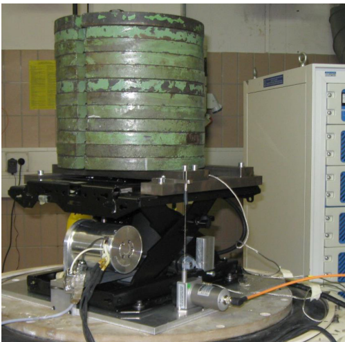
Test set-up of the active driver seat on the shaker
