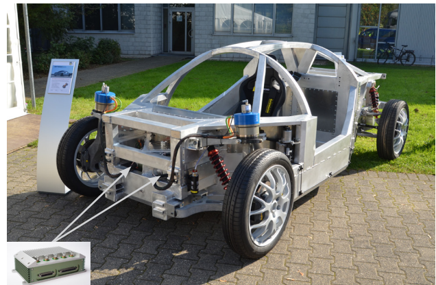
SpeedE with integrated steer-by-wire system
